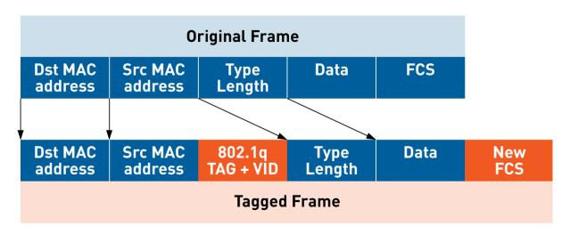
When the original packet matches the TPID fields configured by –1 or –2 parameters, the packets are tagged according to the –ad and VID + port number parameters:
