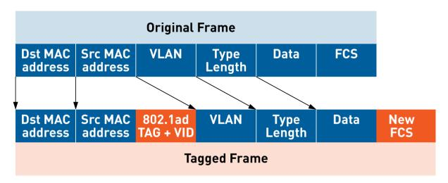
In the case of multiple VLAN present in the original packet, the first TPID field is compared with TPID –1 and –2 parameters. The original VLAN tags are not altered.
